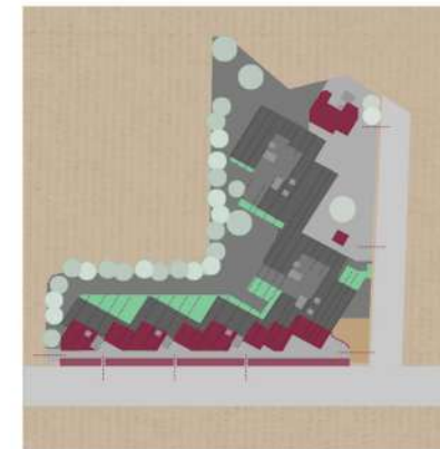
The extroverted public edge is more porous, allowing for multiple access points on the longer edge for commercial spaces. The corner of the site is freed for street vendors. The mandir and cafe are placed on the other edge.
