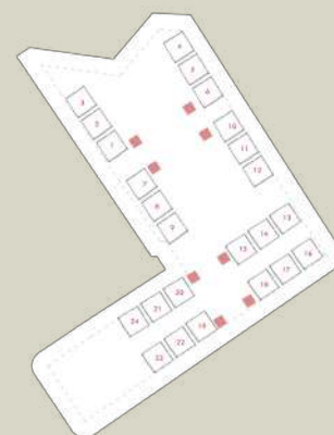
linear organisation which leads to building margin issue in the compact side of the L shaped plot
