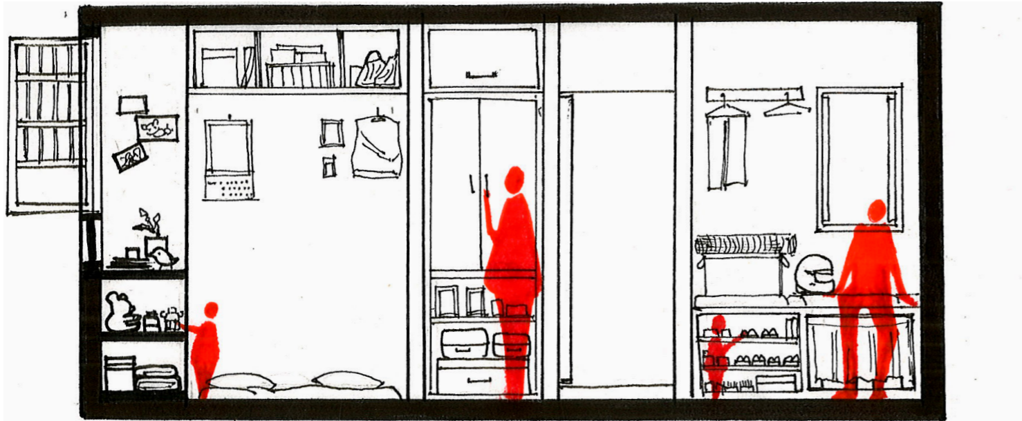
SECTION BB' - Using a mattress for sleeping, frees the floor space for toher activities in the day
